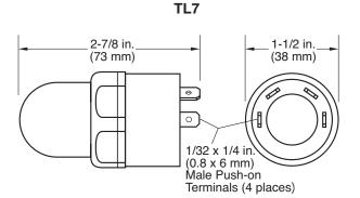
Mounting Hole: 1-1/8 in. (29 mm) diameter Maximum Panel Thickness: 1/4 in. (6 mm)
