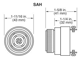
Mounting Hole: 1-1/8 in. (29 mm) diameter Maximum Panel Thickness: 1/8 in. (3 mm)
